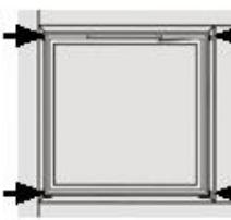
**EN:** Wedge at all corners with temporary wedges (opposing wedges from inside and outside). Side jambs must be vertical and in plane.
