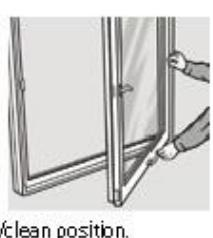
**EN:** Remove sash from the frame as follows:
