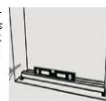
**EN:** Decide and mark the position of the frame in relation to the inner and outer wall.
