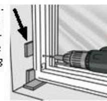
**EN:** Place exactly fitting blocks where the windows fixing holes are positioned, and fix with screws where the predrilled holes are positioned in the frame.
