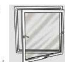
**EN:** b) Close the handles at the bottom, and open the handle at the hinge side, supporting the sash at the same time.
