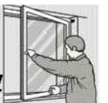
**EN:** Check that the sash on the opening side contacts the frame striking plate at the bottom. There should be gentle contact without having to exert excessive force. Adjust as necessary.
