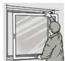
**EN:** Re-fit the sash into the frame by reversing procedure for removal. Open sash to approx thirty degrees in the turn position, and apply reasonable force to the sash to remove any slack in the screws and fixing points.
