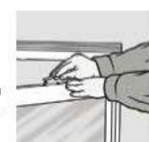
**EN:** The top arm can then be lifted off and the sash removed.
