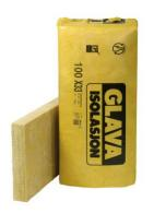
Material: Insulation class: Thermal conductivity: Width: Length: Thickness: Glass wool 33 λ<sub>D</sub> =0,033 W/mK 570 mm and 560 mm 1200 mm Various
