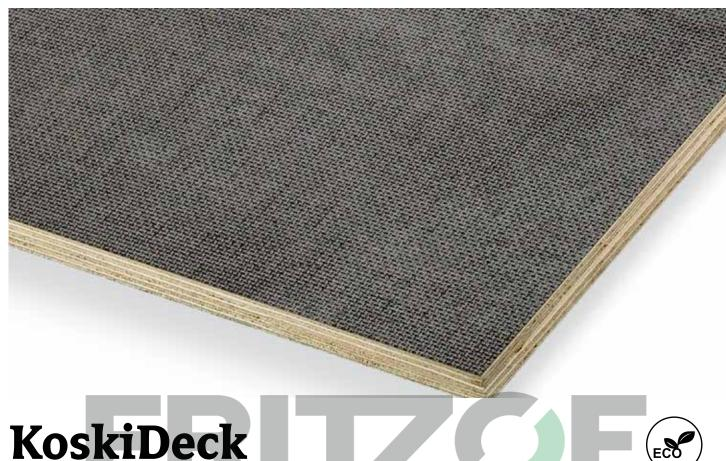
KoskiDeck is Finnish birch or combi plywood coated on both sides with a hard wearing phenolic film overlay. One or two sides are hot pressed with a slip resistant wire mesh
