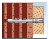
5. Correctly installed anchor in hollow masonry.
