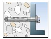
6. Correctly installed anchor in concrete.
