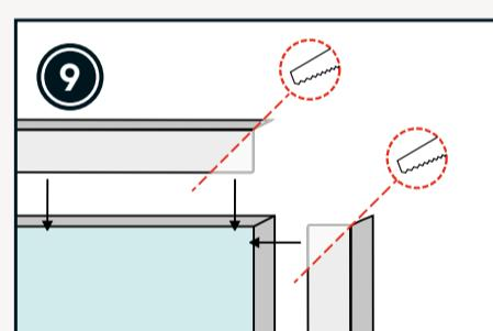
To cover the cut surfaces use an L-profile, cut to length and mitre the corner 45°.
