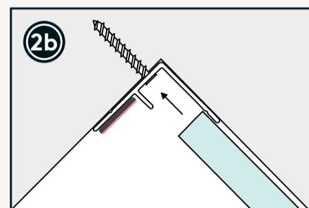
If using the hidden corner profile, this must be screwed to the backwall. Install first panel.
