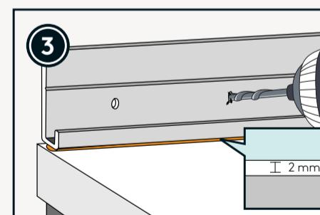
Fasten the bottom list to the back wall about 2 mm above the bench to make room for the sealant.
