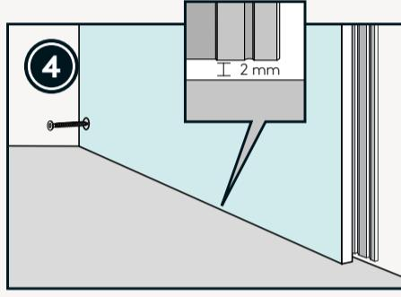
Keep 2-3 mm distance from worktop to bottom of panel. This gap will be filled with Fibo Seal.
