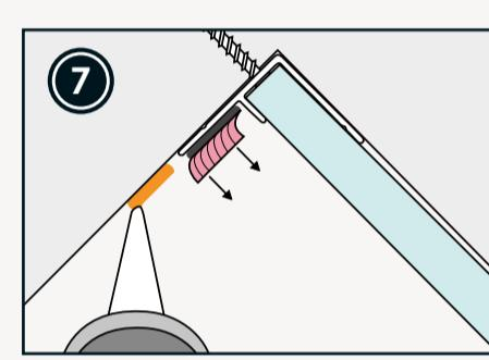
Place a bead of Fibo Seal on the left hand side of the corner profile. Remove protective tape cover on the corner profile before clicking in the last panel.
