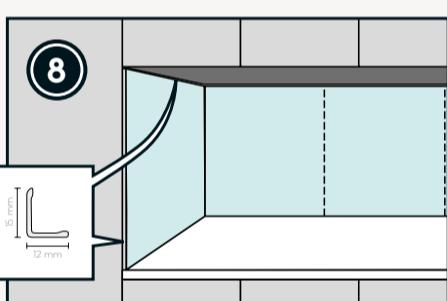
L-Profiles can be used on all cut surfaces to hide screws.
