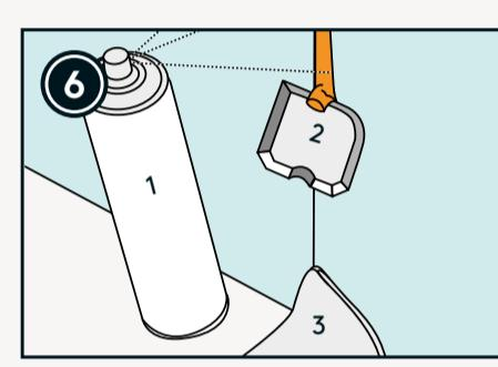
Excess sealant is easily removed by using Fibo Clean and Fibo Sealing Tools. Fibo Wipes can also be used, but soap residue from Fibo Wipes should be removed with paper and water to avoid stains.
