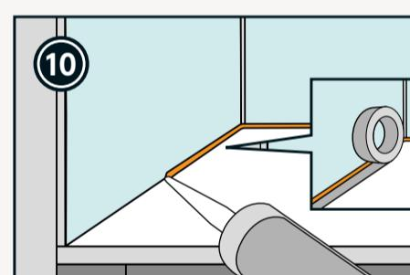
Apply Fibo Seal in the gap between the panels and worktop, and in corners. Masking tape on worktop can be used. Use Fibo Clean and Fibo Sealing Tools for a nice end result.
