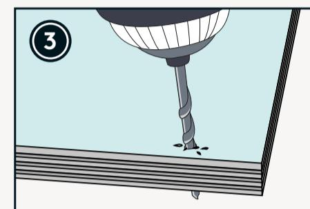
Panel edges to be covered by L-profiles should be pre-drilled for the best result.
