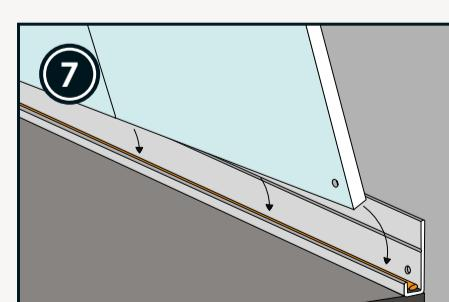
Apply sealant to the base of the bottom profile. Lift the panels collectively and place in the bottom profile. Remove excess sealant.
