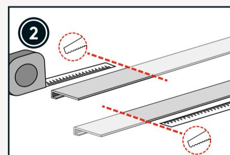
Adjust lenght of bottom profiles. Place a string of Fibo Seal under the bottom list for a waterproof system.
