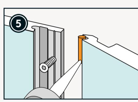
Fasten first panel with Fibo Screws. Apply sealant on the left side of next panel before connecting for a waterproof result.
