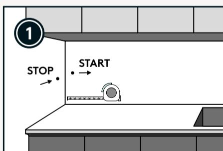
Measure area and adjust panels according to center position and cabinet height if needed.
