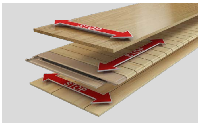
Fig. 1. Cross structure of 3-layer wooden floorboard produced by Barlinek Inwestycje Sp. z o.o.
