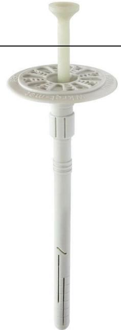
Hammer driven fastener with plastic pin and telescopic design support washer FIXPLUG-8 is made from polyethylene, and the pin from glass fibre-reinforced polyamide which improves its strength. The applied telescopic solution allows for problem-free facing of the support washer and polystyrene surface by its shallow recess. Fastener FIXPLUG-8 should be used to transfer loads of wind suction forces and applied as an additional mechanical fixing for the whole system, recommended for:
