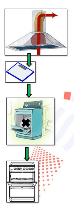
Remove the washable carbon filter from the hood.
